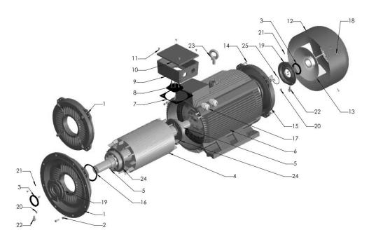
Figure 34: Design of motors from the ACM - AWM - AMY series
