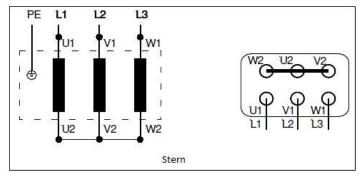
Figure 43: Circuit diagram for forced cooling fan - star
