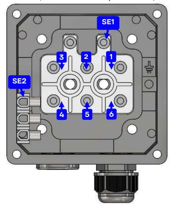
Figure10: Terminal box for ACA, ACM 56 - 132; AFS 80 - 160 three-phase motors
