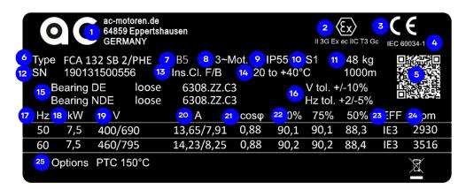
Figure 30: Type plate Ex motor
