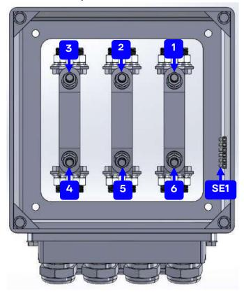
Figure 12: Connection box for three-phase motors AWM 315 - 450
