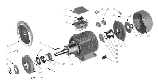
Figure 37: Structure of motors in the AOM series sizes 250 - 355
