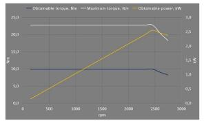
Figure 24: 87 Hz characteristic curve of a 1.5 kW 4P asynchronous motor
