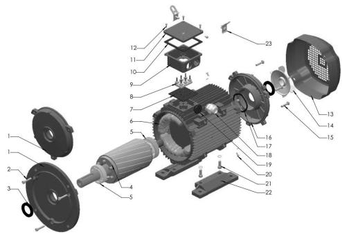
Figure 33: Structure of motors in the ACA - ACY - AFS series
