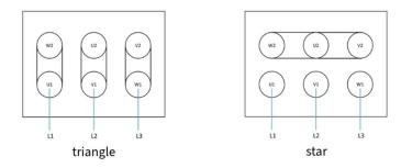
Figure 39: Circuit diagram for single-speed motors
