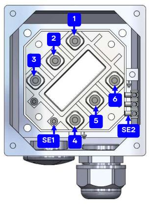
Figure 11: Terminal box for AC motors ACA, ACM, AWM, AMY 160 - 280
