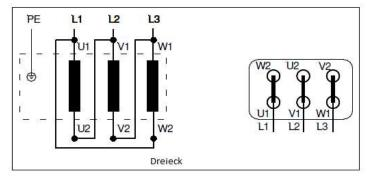
Figure44: Circuit diagram for forced cooling fan - delta
