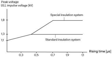
Figure 26: Maximum permissible U<sub>LL</sub> in connection with voltage rise time
