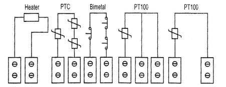
**Figure 42**: Circuit diagrams for standstill heating, temperature sensor PTC - bimetal (PTO) - PT100 (PT1000) 3-wire or 2-wire
