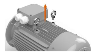
Figure 2: Removing the eyebolts
