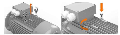
Figure 31: Replacing eyebolts with hexagon head screws for motors with increased IP protection class and Ex motors
