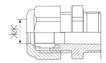
Figure15: Clamping area
