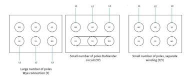
Figure 40: Circuit diagram for pole-changing motors
