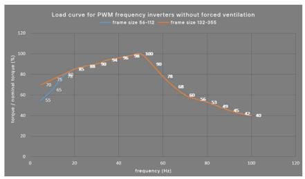
Figure 25: Reduction factor for the torque during operation on the frequency inverter
