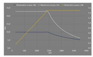
Figure 22: 50Hz characteristic curve of a 1.5kW 4P asynchronous motor
