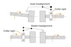
Figure4: axial and radial shaft misalignment
