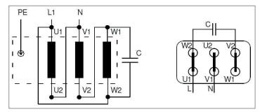
Figure45: Circuit diagram forced cooling fan - 1~
