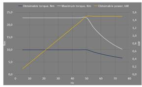
Figure 21: 50Hz - f3 cut-off frequency
