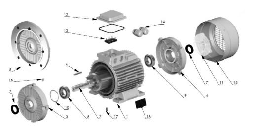
Figure 35: Design of motors in the AOA series sizes 80 - 112
