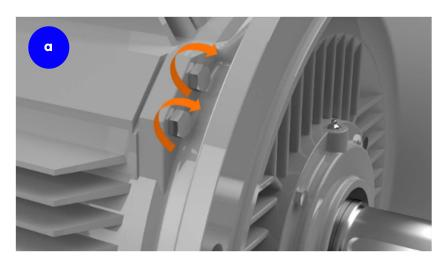
Figure16: Screws end shield
