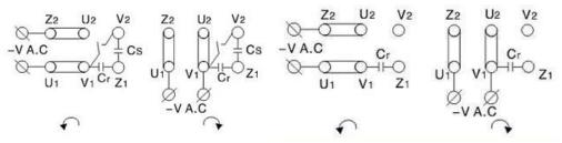
Figure41: Circuit diagram of AC motors
